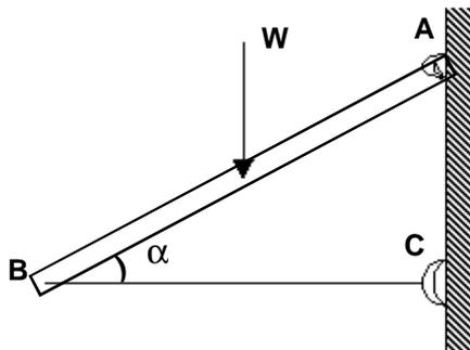
3. (a) A long ladder of length  $L$  supported at  $A$  and  $B$  as shown in fig. A vertical load  $W$  can have any position as defined by the distance "a" from the bottom. Neglecting friction determine the magnitude of the reaction  $R_b$  at  $B$ . Neglect the weight of the ladder. 4
